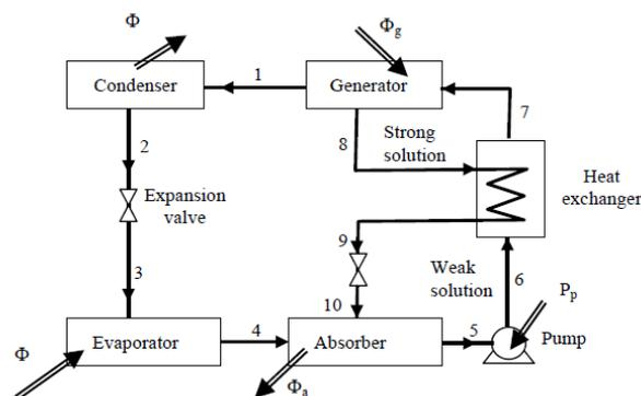
Figure 12 - Schematic representation of adsorption cooling technology..
