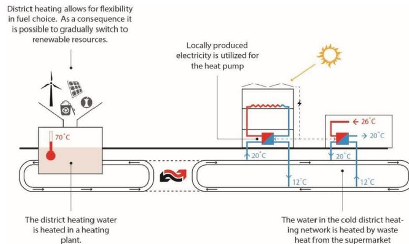
**Figure 9 - Schematic of the interconnection between local and global district heating system.**
