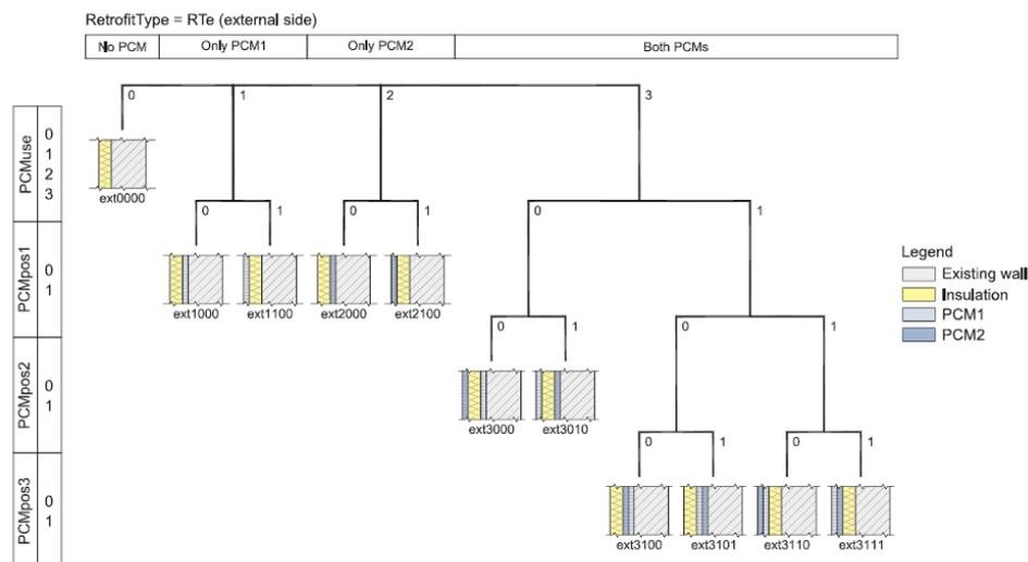
**Figure 18 – Wall configurations for retrofitting on the external side.**
