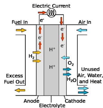
**Figure 14 - Diagram of a PEM-FC (Source: [2]).**
