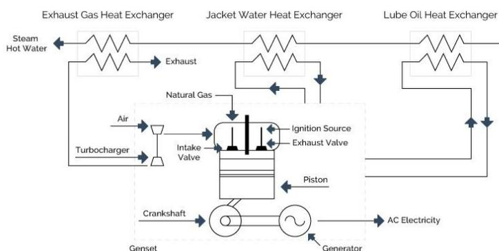
**Figure 11 - Schematic representation of internal combustion engine cogeneration system.**
