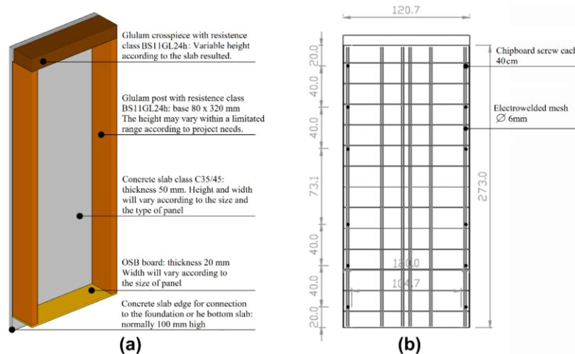
**Figure 3 - CGFP (Concrete Glulam Framed Panel) standard configuration (a) and electrowelded mesh (b) (Source: Boscato, 2018)**
