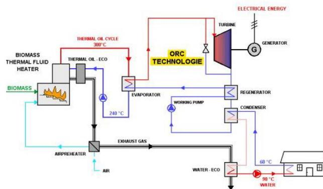
Figure 10 - Schematic representation of biomass cogeneration with ORC technology..
