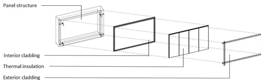
**Figure 4. Schematic of a generic modular panel assembly (Source: adapted from [www.more-connect.eu/](http://www.more-connect.eu/))**
