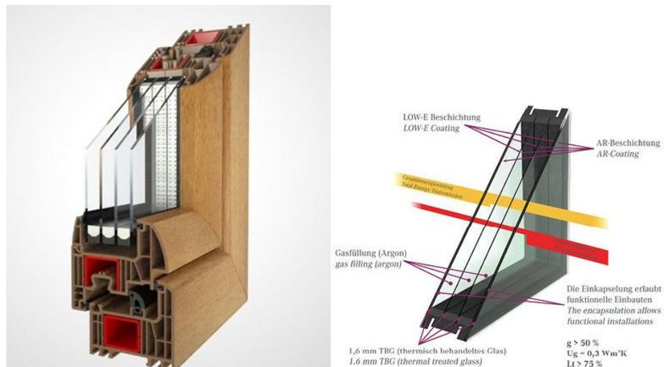
**Figure 2 - Examples of quadruple glazed windows (Source: fenster-Jancic.at left and glaswelt.de right).**
