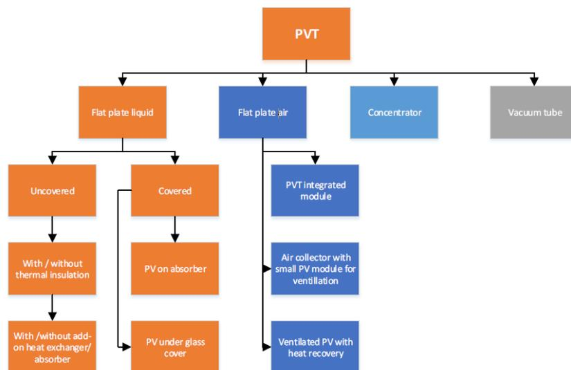
**Figure 13 - PVT Module Classification (Source: [https://www.seac.cc/wp-content/uploads/2018/01/SEAC\\_PVTinSHaPeBenchmark\\_final.pdf](https://www.seac.cc/wp-content/uploads/2018/01/SEAC_PVTinSHaPeBenchmark_final.pdf))**
